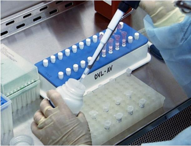
After the specimen has been vacuumed from the extraction column, wash the specimen with 700 microliters of previously prepared RW1 buffer.
