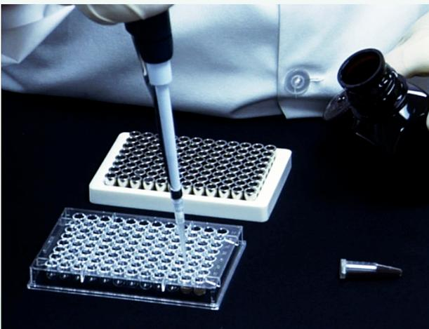
Add 100 microliters of Wash Solution 2. Place the plate on the plate shaker for 30 seconds, then transfer the plate to the magnetic stand before removing the liquid. Repeat the wash step again using Wash Solution 2, the shaker, and magnet.
