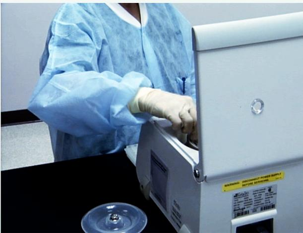
Place the extraction column into the centrifugation tubes supplied with the columns. Dry the column and remove residual ethanol by centrifugation in a microfuge at full speed for two minutes. Note: Residual ethanol is inhibitory to PCR amplification and other down-stream applications.
