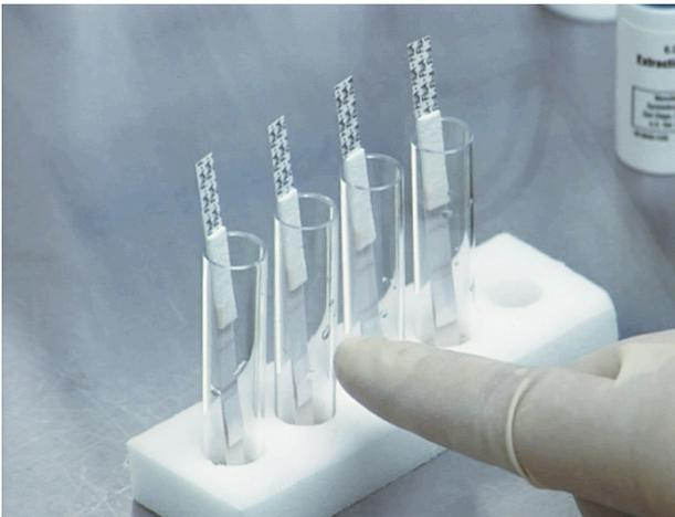
When interpreting results of the test, the top pink line is the control line. If the top pink line develops and the bottom pink line develops at any intensity, the test is positive for type A influenza virus. These specimens show that the first tube from the left is a strong positive, the second tube is a negative, and the third and fourth tubes are both weak positive specimens.
