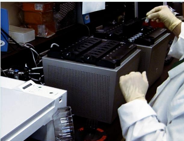
Place the tubes into the Smart Cycler to be tested. Close the Smart Cycler block lids and start the run.
