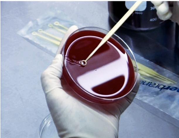
Check the AAF for bacterial contamination by streaking a loopful of AAF onto a blood or nutrient agar plate. Incubate streaked plates for 24 hours at 37°C and record results.
