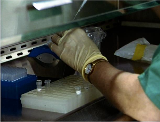
To perform the PCR test on the Cepheid® Smart Cycler, fill the appropriate number of Smart Cycler tubes with 17 microliters of master mix – remembering to keep the hood light off. In addition to the sample tubes, be certain to include two additional tubes, one for a positive and one for a negative control.
