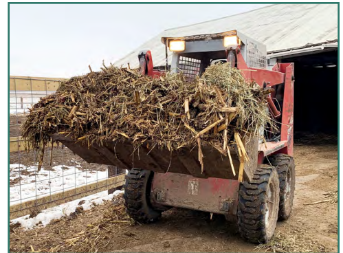
Skid loader used only for manure and soiled bedding handling. Source: Hope Dohman, Iowa State University
