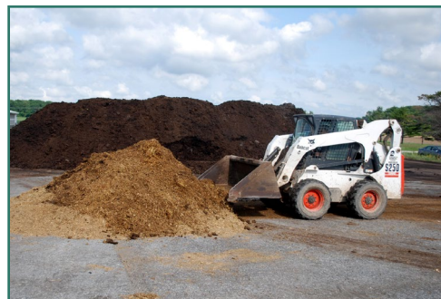
A skid loader is used to cover carcasses in a compost pile. Source: Richard Ehrhardt, Michigan State University Extension
