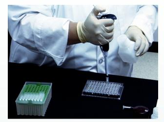
Add 100 microliters of Wash Solution 1 to each well. The Wash Solution will need to be prepared prior to performing the procedure.
