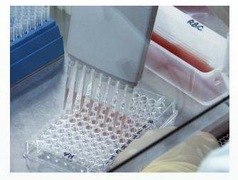
Using nonfiltered, nonsterile pipette tips, add 50 microliters of 0.5% washed erythrocyte suspension to each well. Be sure the erythrocytes are thoroughly suspended and be careful not to allow the pipette tips to come in contact with the sample dilutions to avoid sample carry over.
