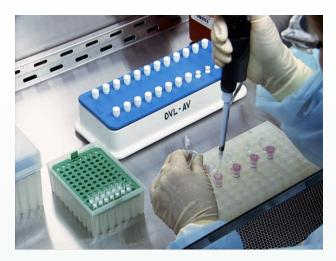
Using sterile pipette tips for each tube, add 50 microliters of RNase-free water to each column. Be certain not to touch the silica-gel membrane of the column with the pipette tip. Incubate the tubes at room temperature for 1 to 3 minutes. Centrifuge the tubes for one minute at 10,000 rpm to elute the RNA. Store the sample at 4° C until the sample is tested. RNA that cannot be tested within 24 hours should be stored at -70° C. Multiple freeze and thaw cycles should be avoided.
