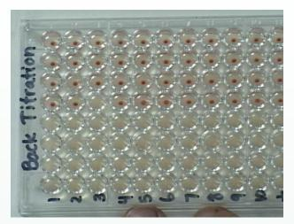
Perform the HA test with the diluted samples using the same procedure as for the HA test. If the appropriate dilutions were made, the endpoint for each sample should be 16 HAUs per 50 microliters as shown in this example.
