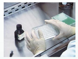
Shake the plate to make sure the lysis/binding solution is thoroughly mixed with the sample.
