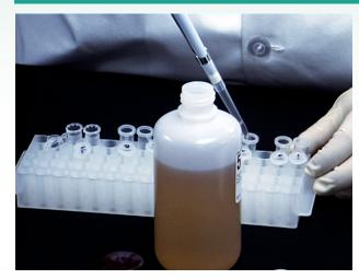
The first step is to dilute the serum samples. The IDEXX kit comes with a dilution buffer. Add 1 milliliter of the dilution buffer to previously labeled dilution tubes. Please note that not every ELISA kit uses the same serum dilution, so be sure to read the manufacturer's instructions carefully for each brand of ELISA kit you use.
