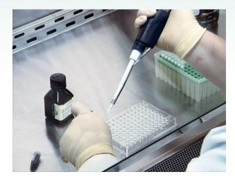
Add 50 microliters of the swab specimen into a corresponding well on a 96 well plate, changing pipette tips between each sample.
