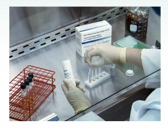
Add one test strip, supplied with the kit, to each specimen tube. Be certain that the pink membrane at the bottom of the strip is completely covered by the solution. Incubate for 15 minutes at room temperature and record test results.
