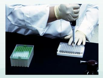
The magnetic beads will migrate towards the magnetic field so that the liquid can be removed with a pipette. Discard the liquid and pipette tips.
