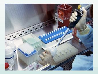
Next, add 500 microliters of RLT lysis buffer to the specimen tube. Do not touch the side of the specimen tube with the pipette tip or insert the tip into the specimen tube. If you do, you will need to change to a new sterile tip.
