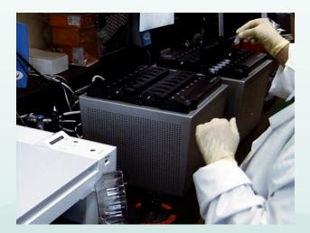
Place the tubes into the Smart Cycler to be tested. Close the Smart Cycler block lids and start the run.
