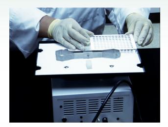
At this point, the virus has been inactivated by the lysis/binding solution so the plate can safely be removed from the biological safety cabinet. Using an orbital shaker, shake the plate on moderate speed for four minutes to mix and suspend the magnetic beads. During this shaking process, the RNA will bind to the magnetic beads.
