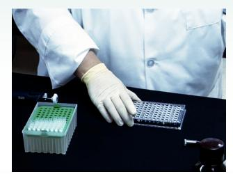
Remove the plate from the magnet so the magnetic beads are released.
