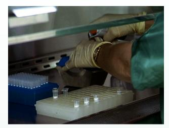
Using sterile pipette tips, add 8 microliters of each RNA sample to a corresponding Smart Cycler tube. Close each tube after adding the RNA. Add 8 microliters of clean water to the negative control tube.
