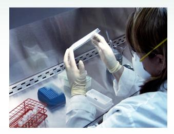
Visually inspect the plate to verify that PBS has been added to the appropriate wells.
