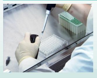
This RNA extraction procedure uses guanidinium thiocyanate, a chemical used to lyse cells and inactivate viruses such as influenza virus. The initial step must be performed in a BSC. Following the addition of the lysis buffer the specimens are no longer infectious and can be safely removed from the BSC.
