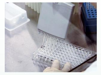
With a single or multichannel pipette set to deliver 25 microliters, make a two-fold serial dilution of the antiserum (in the antigen) across the plate beginning in the first well and continuing through the 8th well. Discard the terminal 25 microliters from the 8th well. At this point each well should contain 25 microliters.
