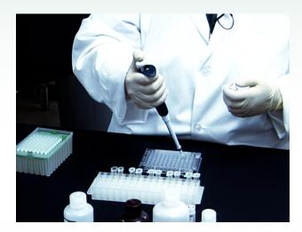
Using the antigen coated plates that come with the kit, start by adding 100 microliters of undiluted negative control serum (provided with kit) into the first two wells (A1 and A2).
