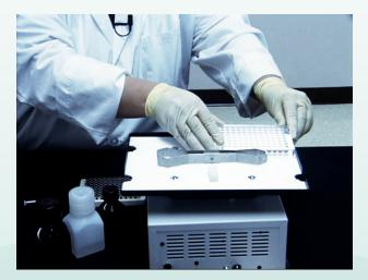
Place the plate back onto the orbital shaker and shake for 30 seconds on moderate speed.
