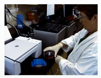
Before you place the tubes in the Smart Cycler, briefly centrifuge the tubes to remove any air bubbles.
