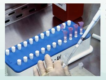
Using an aerosol resistant pipette tip, individually transfer the liquid in each specimen tube to the corresponding extraction column. Note: Care should be taken not to remove or dislodge the pellet from the bottom of the specimen tube.
