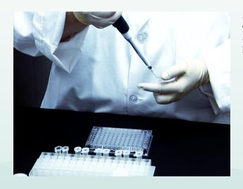
Add 100 microliters of diluted test serum to successive duplicate wells. For example, serum 1 would go in wells A5 and A6, serum 2 would go in wells A7 and A8, and so on. Following the addition of all serums, incubate the plate for 30 minutes at room temperature.
