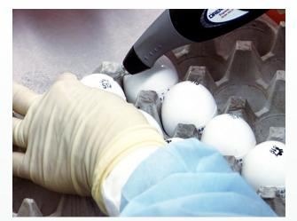
Using a vibrating engraving tool, rotating drill or other suitable tool, drill a small hole just above the air cell.
