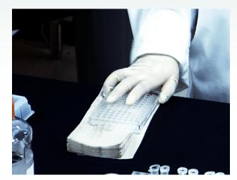
Tap the plate dry on a paper towel to remove all traces of wash solution.
