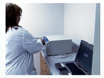
An ELISA reader is used to determine the light absorbency of each sample. Calculate the sample to positive (S/P) ratios by subtracting the average normal control absorbance from each sample absorbance to determine which specimens are positive. Note: Most kits will provide a minimum acceptance value for the positive control that must be achieved for the test to be valid.
