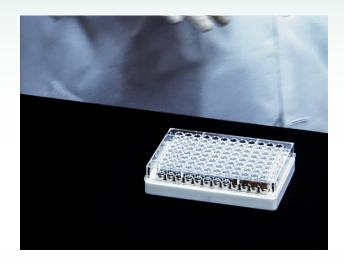
Remove the plate from the shaker and place it on the magnetic stand for one minute.
