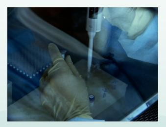
The Probe is light sensitive so you will need to turn off the safety cabinet light before adding the probe to the master mix. Add 6 microliters of the probe that has been diluted to 6 picomoles per microliter. Vortex to ensure uniform mixture, then pulse spin in a microfuge.
