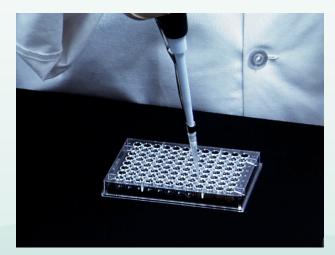
Once the beads appear dry, add 50 microliters of elution buffer to each well then shake on the orbital shaker for 4 minutes.
