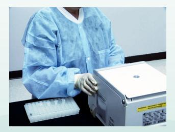
Centrifuge the lysed sample for 5 minutes at 5000 x g to clearify the sample.
