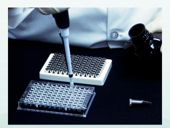
Add 100 microliters of Wash Solution 2. Place the plate on the plate shaker for 30 seconds, then transfer the plate to the magnetic stand before removing the liquid. Repeat the wash step again using Wash Solution 2, the shaker, and magnet.
