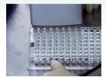
Using a single or multichannel pipettor equipped with non sterile, unfiltered pipette tips, mix the PBS and AAF in the first well of each row. Well contents should be aspirated and expelled (mixed) three to five times to ensure complete mixing. Be sure to keep the pipette tip submerged during mixing to prevent the formation of bubbles.
