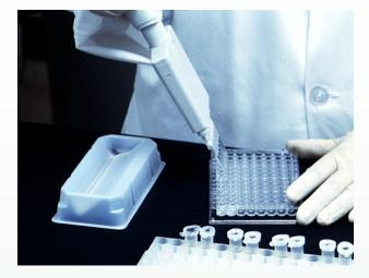
With a 300 microliter multichannel pipette, fill each well with distilled water. Empty the contents of the plate as before. Note: An ELISA plate washer can also be used to perform the washes.
