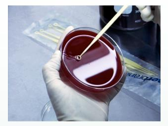
Check the AAF for bacterial contamination by streaking a loopful of AAF onto a blood or nutrient agar plate. Incubate streaked plates for 24 hours at  $37^{\circ}$ C and record results.
