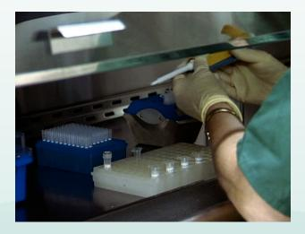
Using a completely different pipette, add 8 microliters of transcribed RNA to the positive AI control tube.
