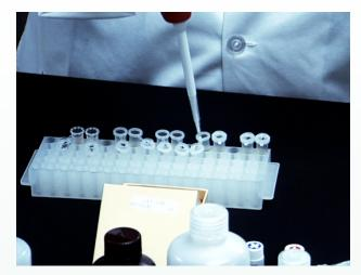
With a sterile pipette tip, add 200 microliters or 0.2 milliliters of each serum to a dilution tube to make a 1:500 dilution of the test serum. Again, not every brand of ELISA uses the same serum dilution.
