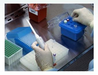
Next add forward and reverse primers, RNase Inhibitor, and enzyme mix. These reagents are perishable so they need to be stored in a refrigerated cooler box until use.
