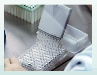
Dispense 50 microliters of PBS to each microtiter plate well being used for the assay, including the positive control row and cell control row.
