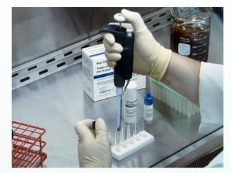
Add 200 microliters of specimen to the corresponding labeled tube. When collecting swabs to use for this test, the manufacturer recommends the use of Brain-Heart Infusion broth (porcine origin).
