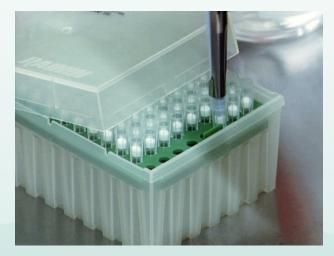
Use a different pipette tip for each sample.
