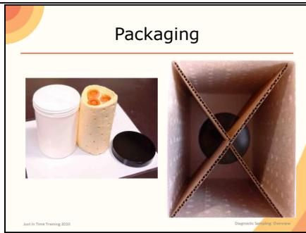
The left photo shows several sample tubes packed in absorbent padding material to prevent breakage and spillage during shipment. These will then be placed in the white plastic container on the left for leak prevention. The right photo shows a shipping box with dividers to keep samples secure during shipping. Photos courtesy of Dr. Dennis Senne, U.S. Department of Agriculture.
