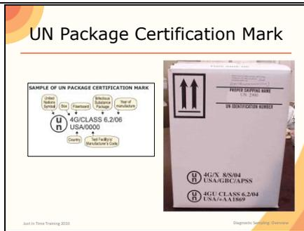
Photos show UN package certification markings required for shipping all infectious substances [CLASS 6.2]. The UN identification number (upper right hand corner of right photo) is required to properly identify the type of sample included in the box. This box is labeled UN2900, containing a Category A, infectious substance, animal only).
